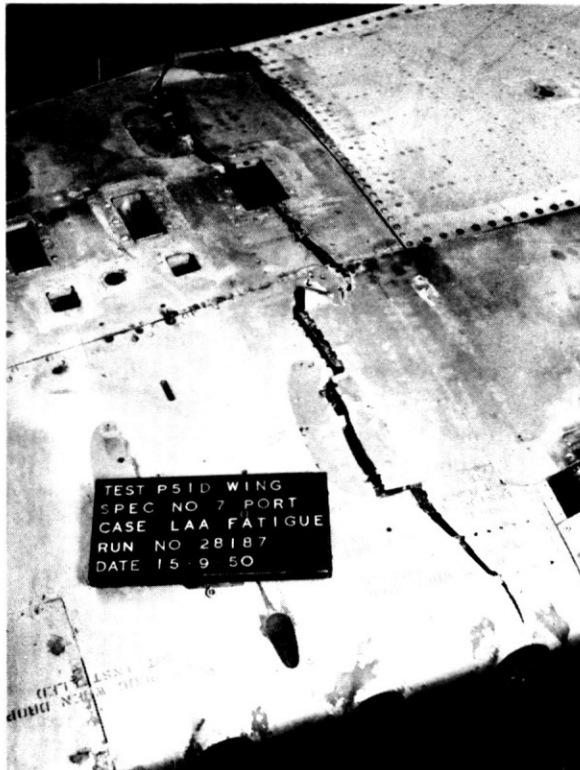
Fig. 2. Fatigue failure at Station 80—Type I.
